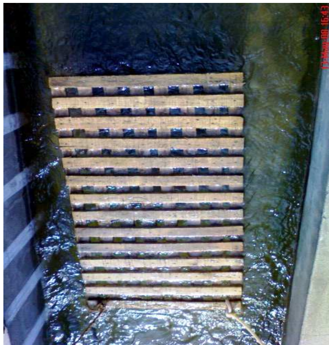
Ankur holding the instrument in position. Notice the wooden wave suppressor used.
